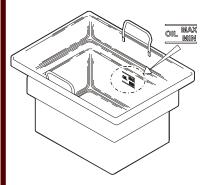
Fig. 5 Oil Level Marking
